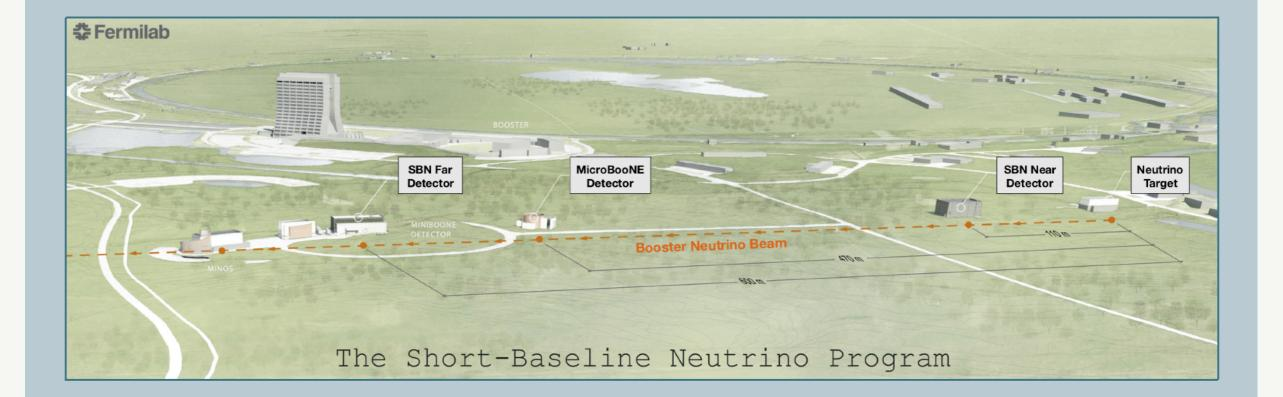
Three detectors: SBND (100 m), MicroBooNE (470 m) and ICARUS (600 m)
